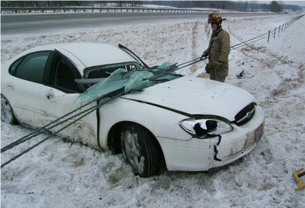
Figure 54. Diving Potential Underride Penetration Crash on Nucor NU-CABLE Barrier
