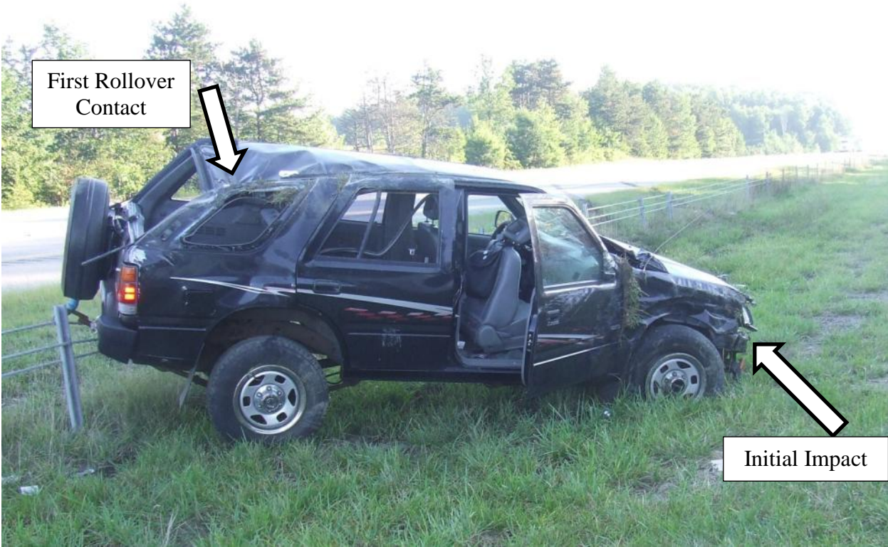
Figure 75. Example Rollover Crash Caused by High Orientation Angle at Impact
