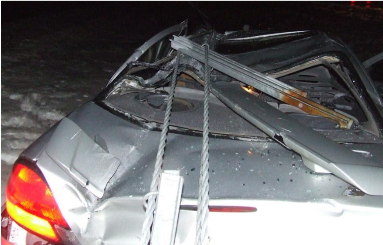
Figure 52. Potential Penetration Crash on Nucor NU-CABLE Barrier
