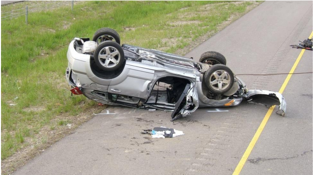
Figure 70. Example Rollover Crash Caused by High Redirection on Back Slope
