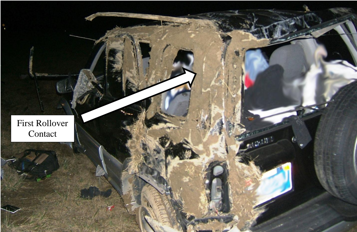
Figure 74. Example Rollover Crash Caused by High Orientation Angle at Impact
