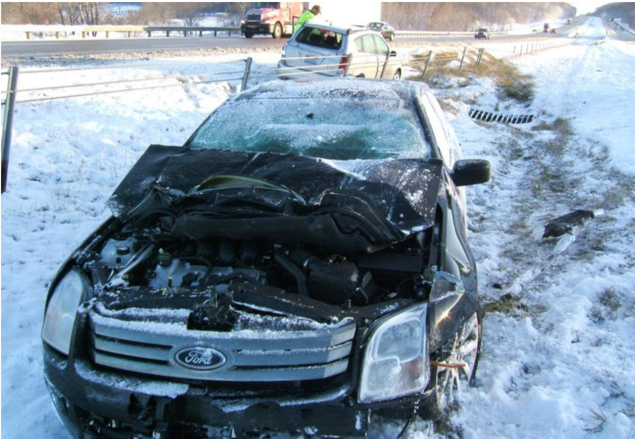
Figure 53. Diving Underride Penetration Crash on Nucor NU-CABLE Barrier
