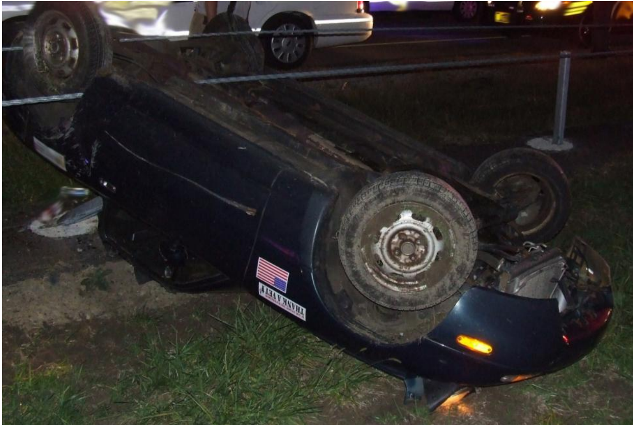
Figure 77. Example of Post Snag Rollover Crash
