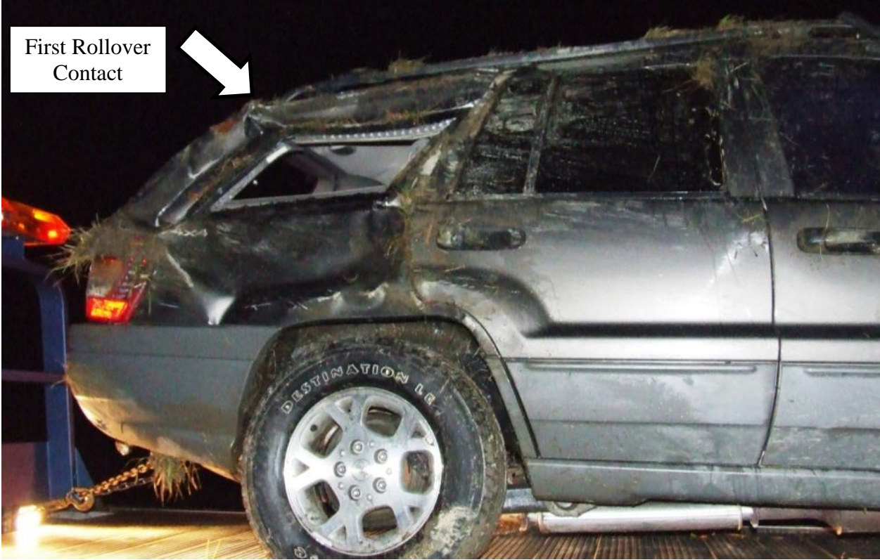
Figure 73. Example Rollover Crash Caused by High Orientation Angle at Impact
