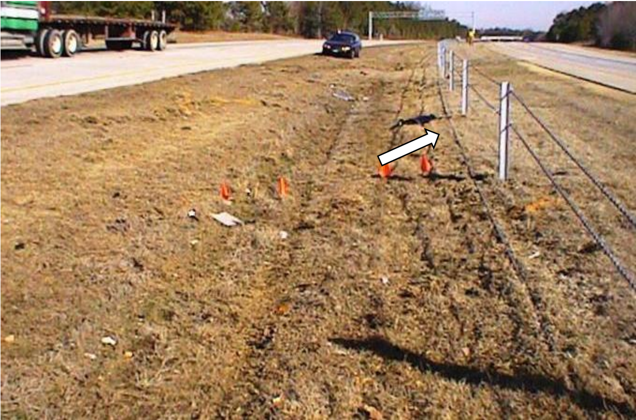
Figure 64. Middle Cable Release from 11 Downstream Posts Resulting in Penetration
